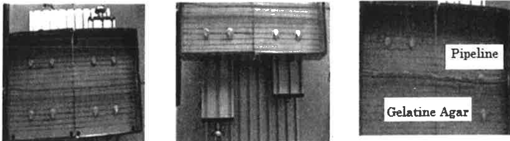
Fig. 4.3 Experiment device for fault dislocation in horizontal movement
